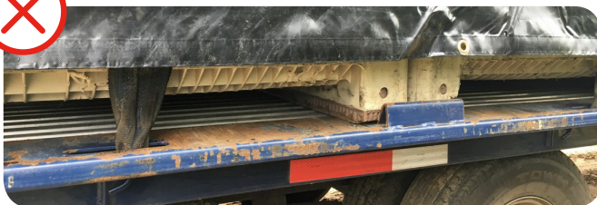
Tarping must be down to the truck bed.
